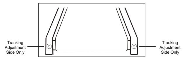
Note: Adjustment is thru small hole of end cap.
