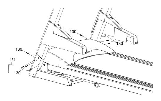
**Step 4.**Install the Frame Base Cap (#61 & #62) on the Frame Base (#2) with the 6pcs of 5x16mm sheet metal Screws (#120) by using the Combination M5 Allen Wrench & Phillips Head Screw Driver (#131).
