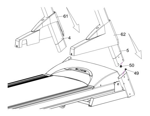
**Step 3.**Install the upright tubes (#4 & #5) into the Frame Base (#2) with the 8pcs of 5/16"x1/2" Button Head Socket bolts (#130) by using the Combination M5 Allen Wrench & Phillips Head Screw Driver (#131).
