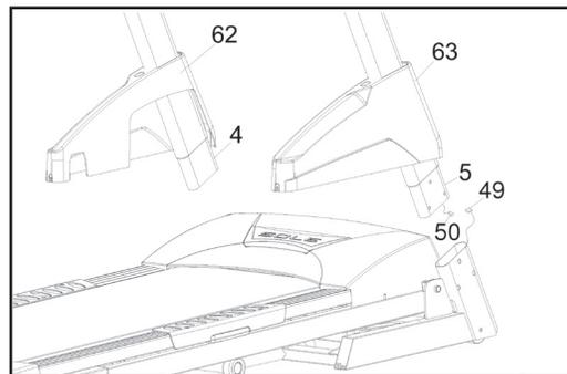
**Before attaching the hardware to Step 3, make sure the cables you just connected don't get pinched in between the steel tubing. If they do, this may cause issues that prevent the treadmill from operating properly.**
