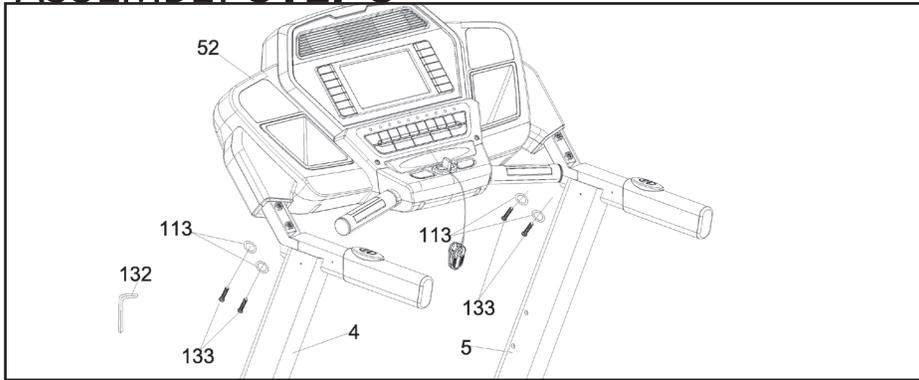
1. Attach the Console Assembly (52) onto the Upright Tubes (4 & 5) and attach with four Button Head Socket Bolts (133) and four Split Washers (113). Tighten using the M6 Allen Wrench (132). Tighten completely.
