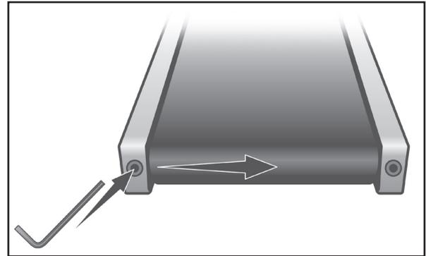
Continue to make 1/4 turns until the belt stabilizes in the center of the running deck.
