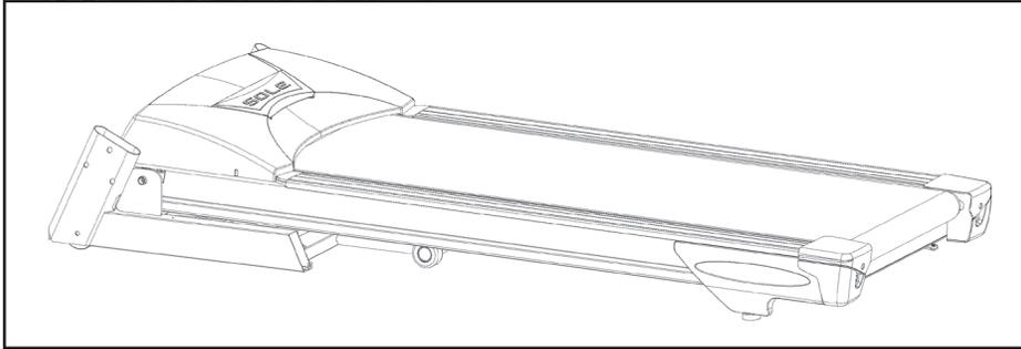
1. Remove the treadmill from the carton and position it aside on a smooth, level floor. The rear should be at least 3' from any wall. Do not remove the Velcro belt until you have removed the plastic wrap and Styrofoam from beneath the unit. **Turning the unit on its side after removing the belt may cause the unit fold up and cause serious injury!**
