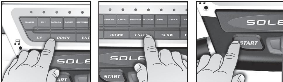
2. If enter was pressed, the **Message** window will display **Age**. You may use any of the **Up/Down** or the **Fast/Slow** keys to adjust your age. After adjusting press the **Enter** key. (**Note:** You may press start at any time during the programming to start the program with the information you've already input.)
