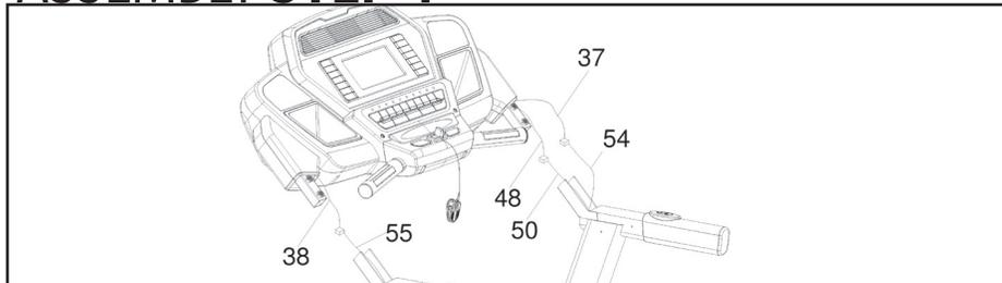
To complete this step, it is recommended that you find something to rest the console on at the appropriate height or have someone hold the console while you connect the cables
