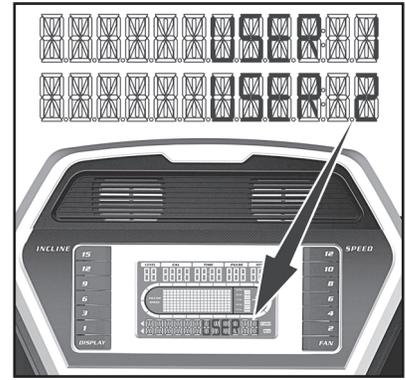
2. Next the **Message** window is flashing **Age**. Use the Adjust **Up/Down** keys to adjust. Press **Enter**. This is a must to continue even if age is not adjusted.
