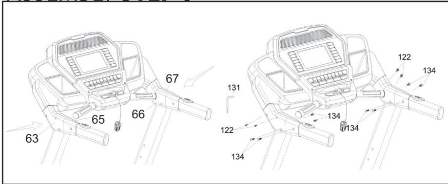
1. Attach the Left (63 & 65) and Right (66 & 67) Side Caps to the top of the Upright Tubes (4 & 5) with eight Phillips Head Screws (134) and four Sheet Metal Screws (122). Tighten with the Combination M5 Allen Wrench & Phillips Head Screw Driver (131). See illustration to determine the specific screw locations.
