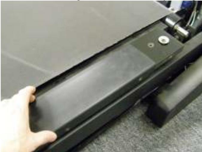
5. Using an allen wrench, remove the 4 deck bolts.
