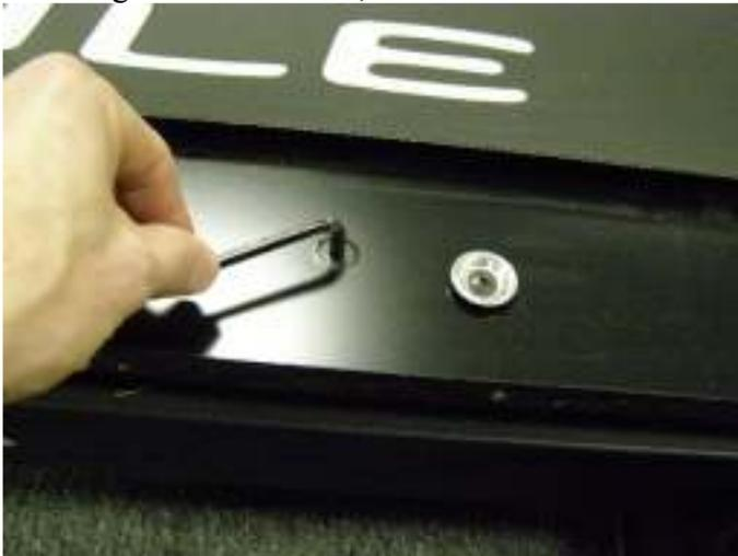
6. Using an allen wrench, loosen the walking belt. Turn the bolts on each side, counter-clockwise 10-15 turns.
