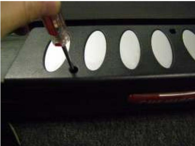
4. Remove the two pieces of the footrail by sliding them toward the end of the treadmill.
