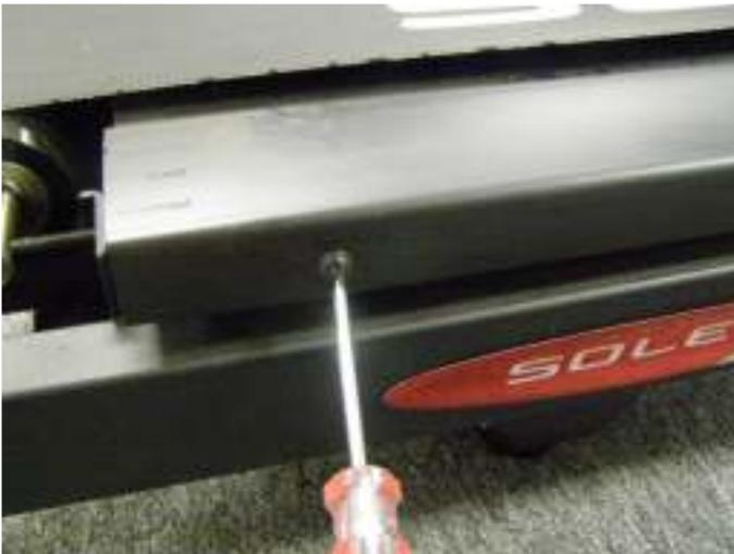
3. Remove the 3 screws that hold down the footrail cover and remove the cover.
