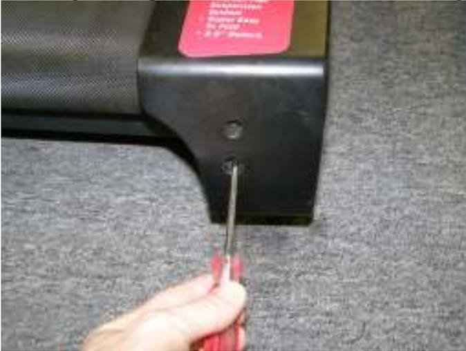
2. Remove the 4 screws on the side of the footrail.
