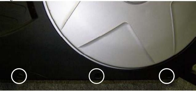
2. Once these 6 screws are loose, you will be able to slide the covers forward or backward in order to stop the disc from rubbing.
