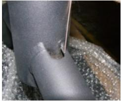
3. Pull the wire and cable all the way through. Loop the wire and run it back into the end of the handle and out through the large hole in the grip.
