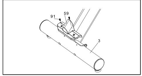
1. Attach the Rear Stabilizer cover with two Screws (**91**). Tighten using the Combination M5 Allen Wrench & Phillips Head Screw Driver (**86**).
