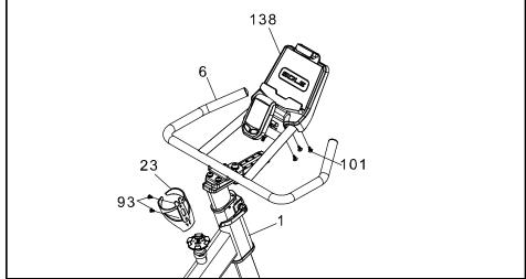
1. Install the Tablet Holder (138) on the Handlebar (6) with 3pcs of Sheet Metal Screws (101) by using the M5\_Combination M5 Allen Wrench & Phillips Head Screw Driver (86).
