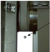
3. Remove base caps on right and left with a Phillips screw driver. (bottom hole)
