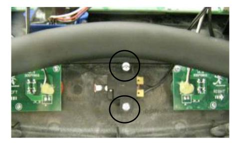
3. Unplug the safety key module from the display board. The board will say "SAFETY" beside the plug.
