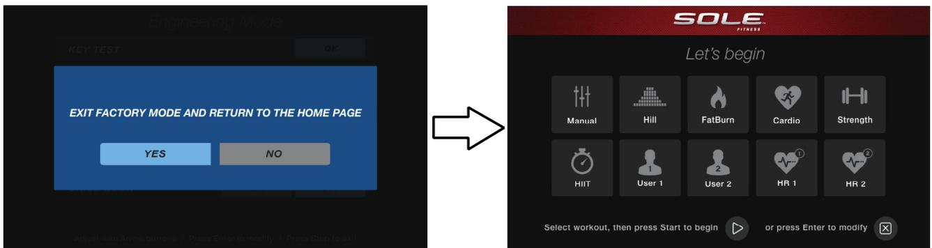
**Incline Calibration:** If there is a problem with the incline, try running the calibration. Press the Incline up key and the Start key at the same time. Hold them down for 5 seconds and press Start key to begin Incline calibration will start and run automatically. Exit the calibration page you need to power off then power on. If the problem persists contact service department.
