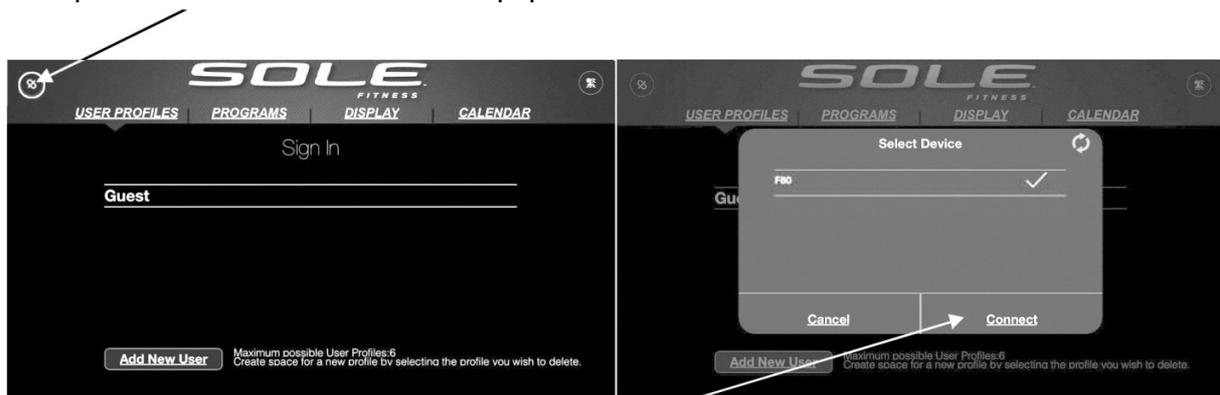
After the equipment is detected, tap Connect. When the App and equipment are synced, the Bluetooth® icon on the equipment's console will light up. You may now start using your new Sole product!
