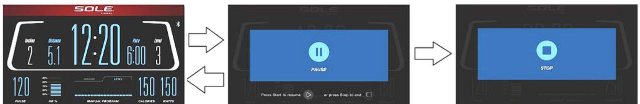
2. When the program ends the Window will show a summary of your workout. The summary will be displayed for a short time then the console will return to the startup display. SUMMARY data contains TIME, DISTANCE, CALORIES, AVG. PACE, and AVG. RPM, and AVG. SPEED, and AVG. RAMP and the AVG. LEVEL, AVG. WATTS, AVG. PULSE.
