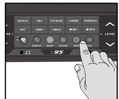
If the **Stop** key is held down for 3 seconds the console will perform a complete **Reset**. During data entry for a program the **Stop** key performs a **Previous Screen** function. This allows you to go back one step in the programming each time you press the **Stop** key.
