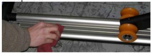
2. Using the lube that came with your machine, you need to lightly coat the rails and wheels with lube.
