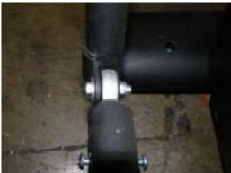
3. Remove the carriage bolt that is under the pedal that holds the connecting arm to the pedal arm.
