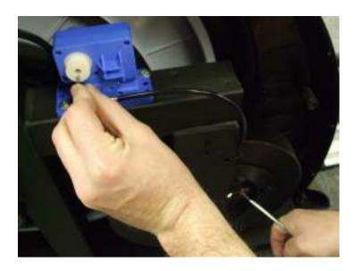
Step7. While holding the slide that brake cable hooks into in flywheel to the left, attach the brake cable to new gear motor. After cable is attached you will want to test to make sure it is working properly. To test the resistance you will need to run the resistance to the max, and back down to the lowest level.
