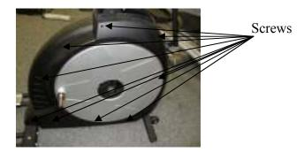
Step1. First you want to go to the right side of the machine and remove the ten screws that hold chain covers together.
