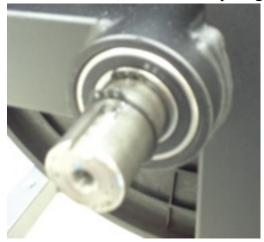
8. Slide axel out from the right side and put spacer in place.
