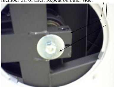
5. Loosen nut that tensions the drive belt. (It may help to loosen this nut)
