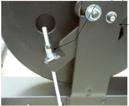
6. Once the belt is loose, slide it off of large pulley.
