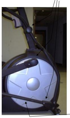
2. Remove these <u>two bolts</u>. Remove <u>swing arm</u>, <u>connecting arm</u>, and <u>step arm</u> all in one piece. Repeat on other side.
