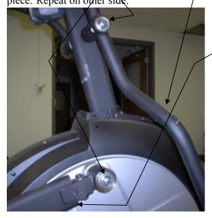
3. Take off right and left chain covers. There should be 10 screws on the right side and 4 that hold the left side on (3 on the bottom and one on the right side near the mast).
